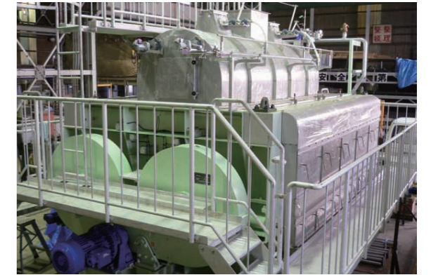
Double Drum Dryer \phi 1,600 \times 4,000L
