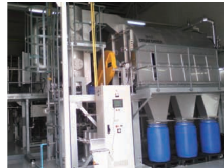
Single Drum Dryer with dual-roll (Waste water drying system) φ1,000 x 1,500L
